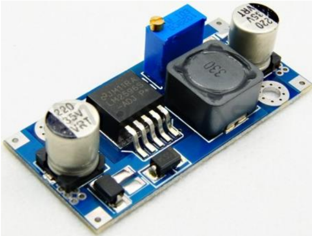
Figure 4-16 4015Step-Down Voltage(12v to 5v)
